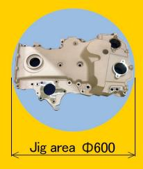
Consolidation of machining processes for large aluminium workpieces using a tilting NC rotary table equipped with a roller gear cam mechanism
