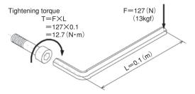
• Tightening torque is moment of force when you tighten a bolt. Tightening torque= FXL.
