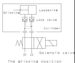
The gripping position must be retained.
