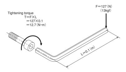
• Tightening torque is moment of force when you tighten a bolt. Tightening torque= FXL.
