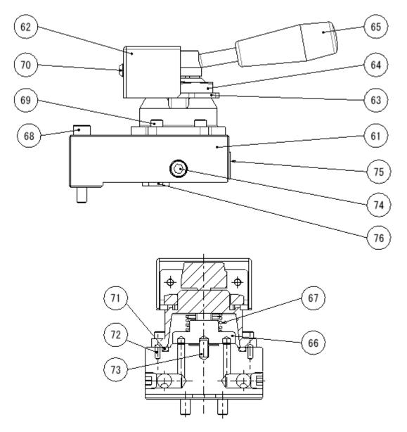
Fig6. Manual operated valve
