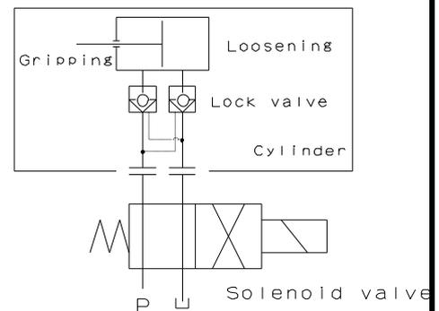
The gripping position must be retained.
