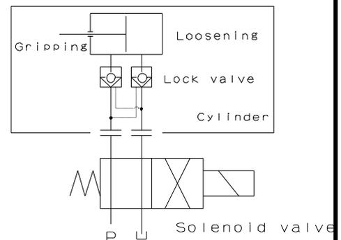
The gripping position must be retained.
