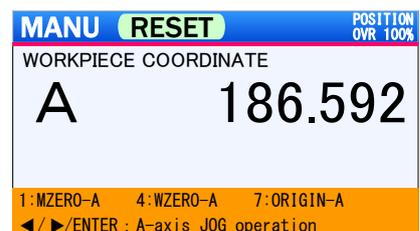
6. When performing a workpiece origin setting of the A-axis, the **7** key is pressed, workpiece origin setting confirmation popup appears.
