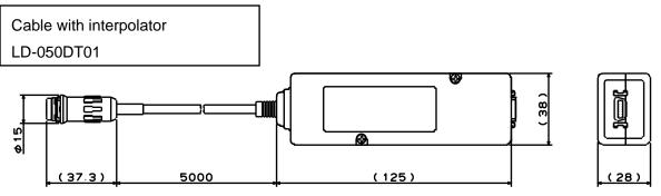
Output connector: 10214-52A2PL manufactured by 3M (MDR connector receptacle)
