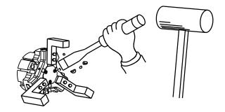
If using the gripper as a workpiece fixture when the workpiece is drilled, deburred, welded, or modified additionally, confirm the specifications. If the gripper is used out of the specifications, not only the gripper is damaged but also the fixed workpiece may fly out.
