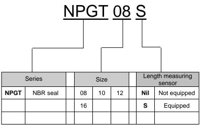
\* For the gripper equipped with the length measuring sensor, see also the separately provided instruction manual for it.
